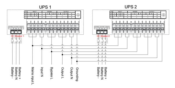
Figure 3-31 11 mode parallel system wiring diagram of 10/10S/10T/15/15S/15T/20/20S/20T
