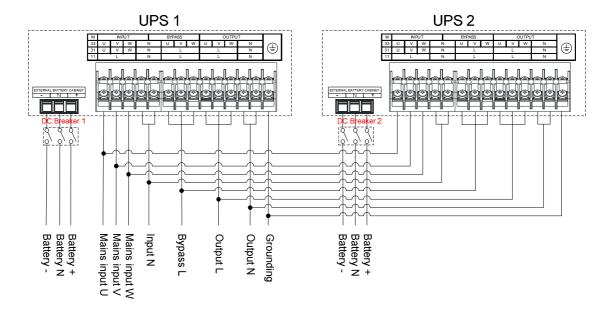
Figure 3-30 31 mode parallel system wiring diagram of 10/10S/10T/15/15S/15T/20/20S/20T
