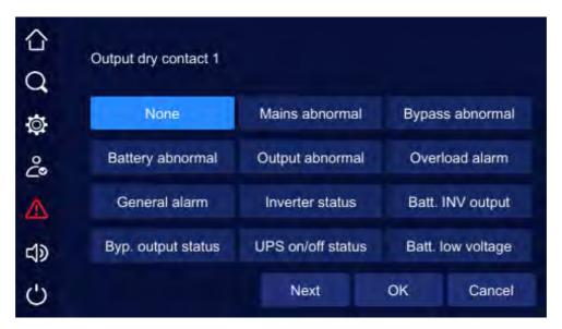
Figure 5-37 Output dry contact setting page 2
