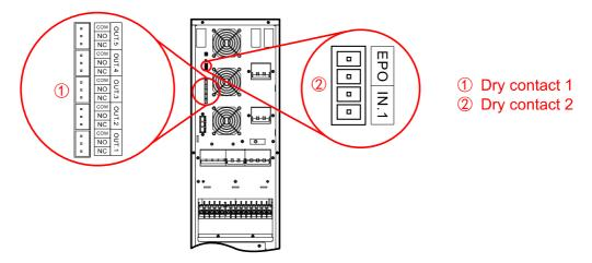
Figure2-10 Dry contact position of 10/10S/10T/15/15S/15T/20/20S/20T
