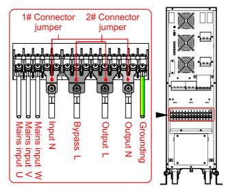
Figure 3-15 Connector jumper and wiring diagram of 31 mode
