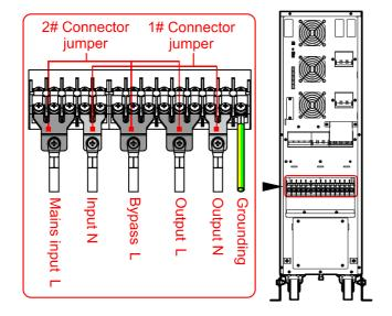
Figure 3-16 Connector jumper and wiring diagram of 11 mode
