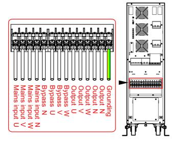
Figure 3-13 Wiring diagram of 33 mode
