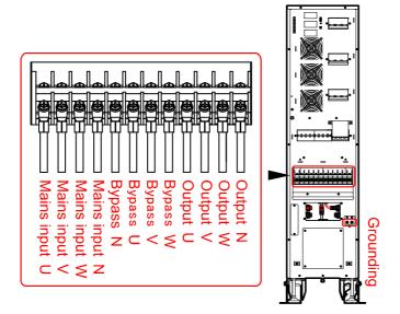
Figure 3-21 Wiring diagram of 33 mode
