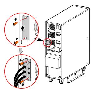
Figure 3-28 Extension battery wiring assembly of 10kVA
