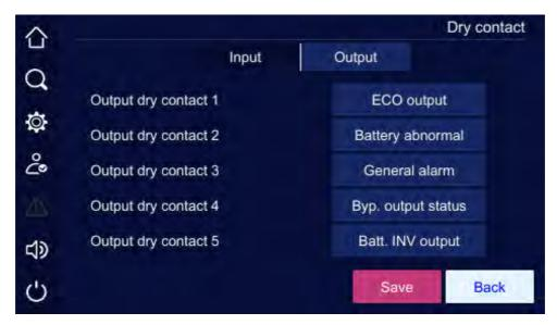
Figure 5-36 Output dry contact setting page 1
