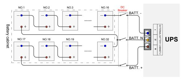
Figure 3-25 Wiring diagram 1 of external batteries
