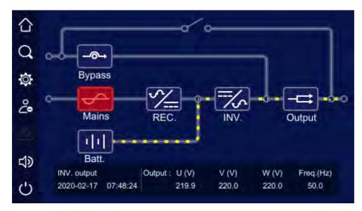
Figure 5-5 Mains abnormal, battery inverting status
