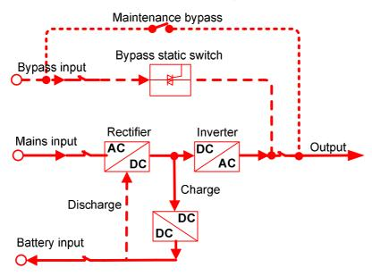
Figure 2-13 Normal mains power supply mode (the thick solid line stands for the energy flow direction)
