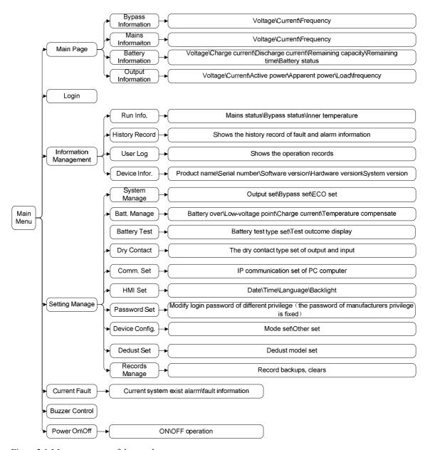
Figure 5-1 Menu structure of the touch screen
