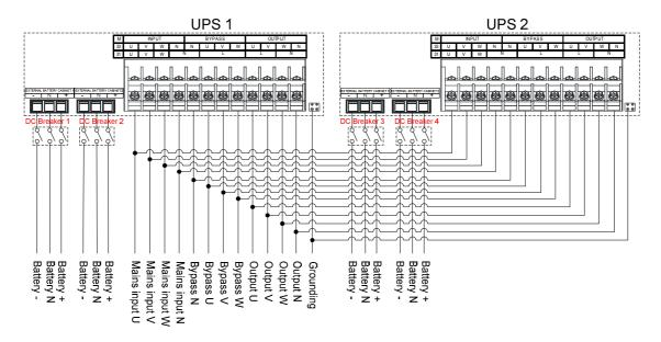
Figure 3-32 33 mode parallel system wiring diagram of 30/30S/30T/40/40S/40T
