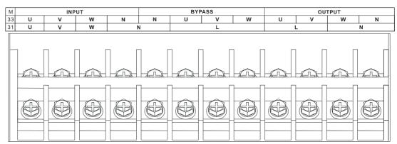
Figure 3-19 Wiring terminal silk-screen
