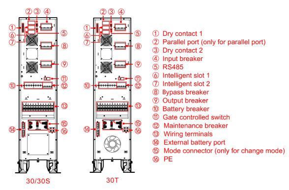
Figure 2-8 Structure of 30kVA rear panel
