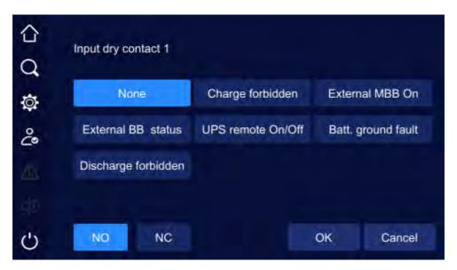
Figure 5-35 Input dry contact setting page 2
