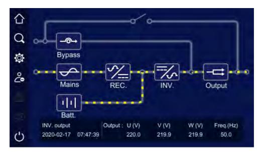
Figure 5-4 Mains normal, mains inverting status
