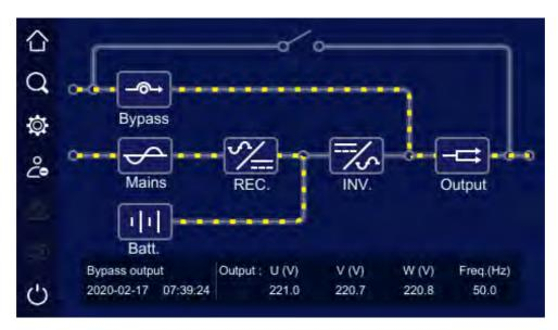
Figure 5-6 Bypass output status
