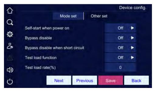
Figure 5-42 Mode set page 2 of device configuration
