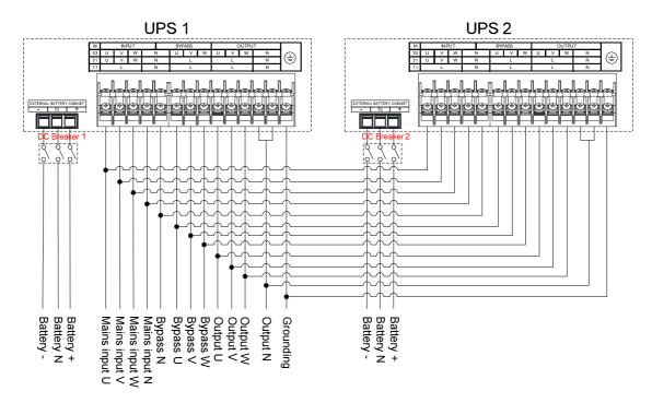
Figure 3-29 33 mode parallel system wiring diagram of 10/10S/10T/15/15S/15T/20/20S/20T
