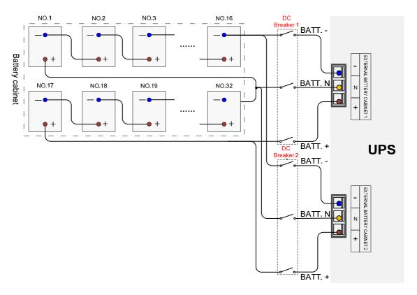
Figure 3-26 Wiring diagram 2 of external batteries
