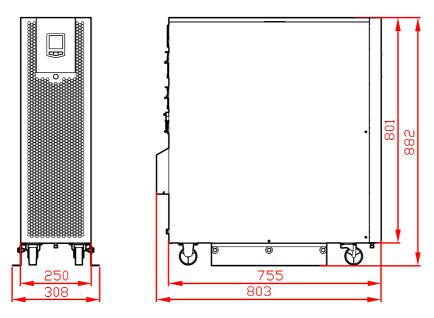
Figure 3-6 Outer dimensions of UPS 10/10S/10T/15/15S/15T/20/20S/20T (unit: mm)
