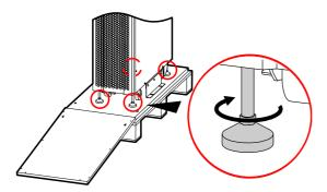
Figure 3-5 Screw up the supporting feet brackets
