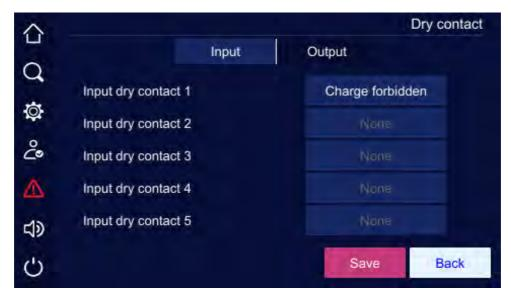
Figure 5-34 Input dry contact setting page 1
