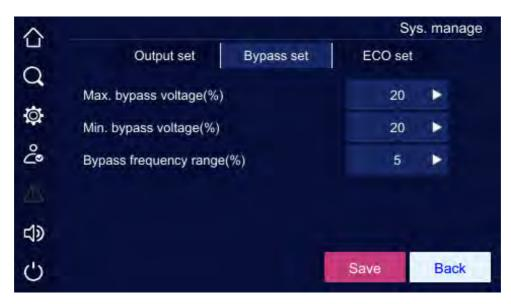
Figure 5-25 System manage page 2 of bypass set
