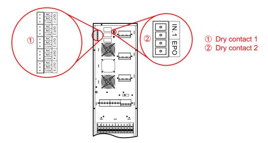
Figure2-11 Dry contact position of 30/30S/30T/40/40S/40T
