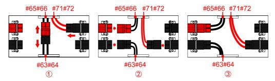
Figure 3-23 Mode connector diagram of 31 mode
