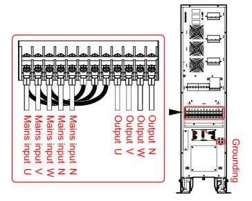
Figure 3-22 Wiring diagram of 33 mode
