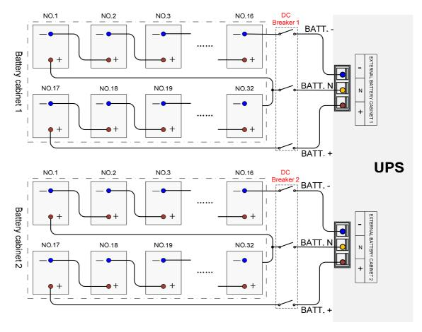
Figure 3-27 Wiring diagram 3 of external batteries
