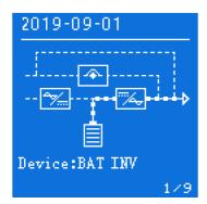
Figure 4-4 Battery inverter output
