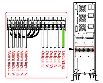
Figure 3-14 Wiring diagram of 33 mode
