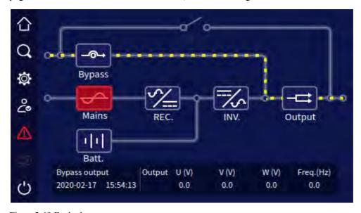
Figure 5-49 Fault alarm status
