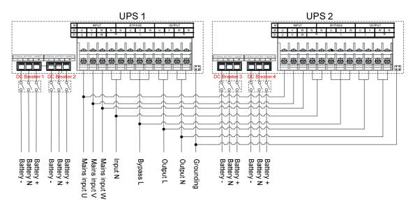
Figure 3-33 31 mode parallel system wiring diagram of 30/30S/30T/40/40S/40T
