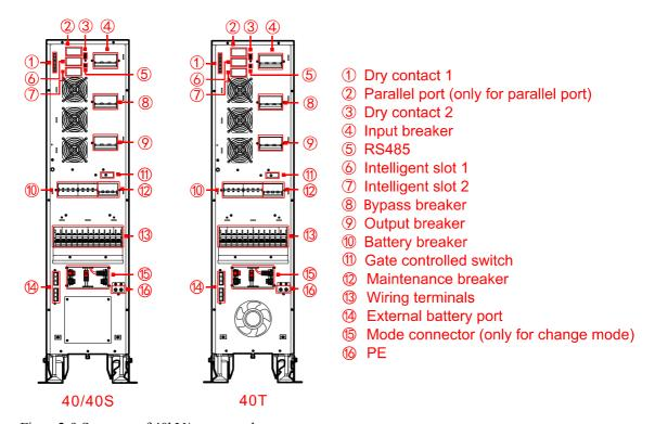
Figure 2-9 Structure of 40kVA rear panel
