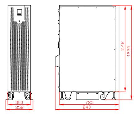
Figure 3-7 Outer dimensions of UPS 30/30S/30T/40/40S/40T (unit: mm)
