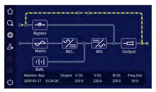
Figure 5-8 Maintenance bypass output status
