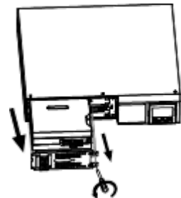
Pull out the battery box by removing two screws on the front panel.
