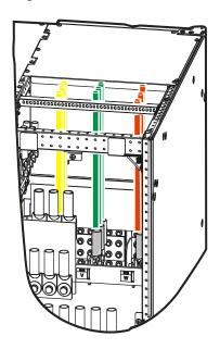
Figure 3-28 The PS500KVA . PS600KVA bypass input wiring diagram
