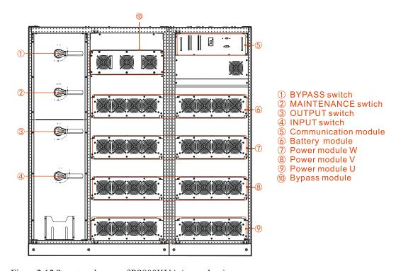
Figure 2-12 Structure layout of PS800KVA (open door)
