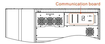
Figure 3-34 Communication board of PS500KVA, PS600KVA
