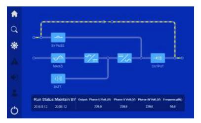
Figure4-11 Maintenance bypass output status
