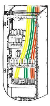
Figure 3-39 The PS800KVA AC input wiring diagram
