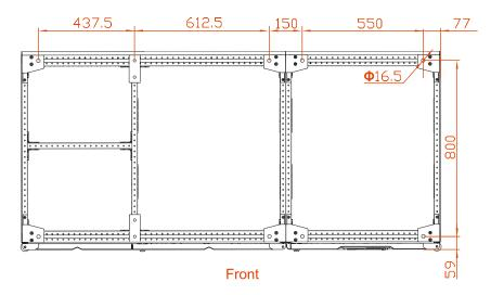
Figure 3-13 Pedestal installation size of PS800KVA (unit: mm)
