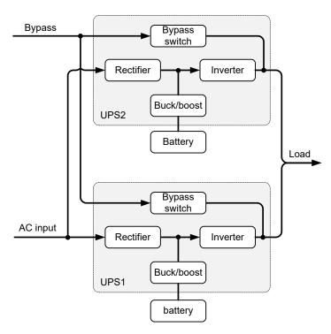
Figure 2-4 Operating principle of parallel system
