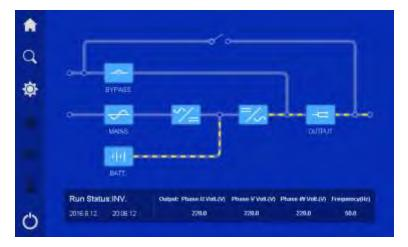
Figure 4-7 Mains abnormal, battery inverting status
