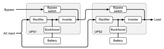
Figure 2-3 Operating principle of series hot-standby system
