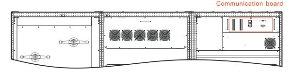
Figure 3-47 Communication board of PS1000KVA, PS1200KVA
