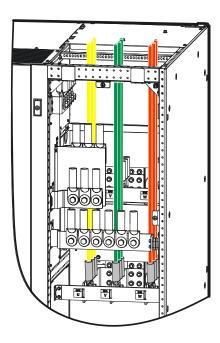
Figure 3-29 The PS 500 KVA \, PS 600 KVA AC output wiring diagram
