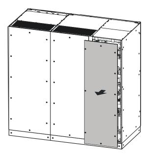
Figure 3-35 Dismantle wiring cover plates of PS800KVA
