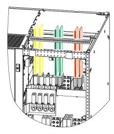
Figure 3-37 The PS800KVA bypass input wiring diagram
