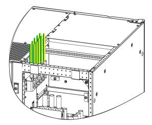
Figure 3-31 The PS500KVA, PS600KVA grounding wiring diagram
