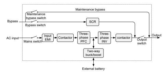
Figure 2-2 Operating principle of single-unit
