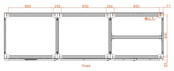
Figure 3-14 Pedestal installation size of PS1000KVA PS1200KVA (unit: mm)
