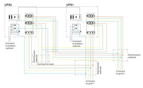
Figure 3-50 Parallel system's wiring diagram
