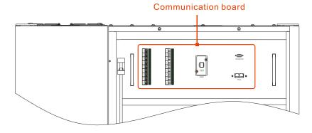
Figure 3-25 Communication board of PS300KVA, PS400KVA
