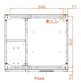
Figure 3-11 Pedestal installation size of PS300KVA, PS400KVA (unit: mm)
