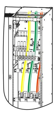
Figure 3-30 The PS 500 KVA \, PS 600 KVA AC input wiring diagram
