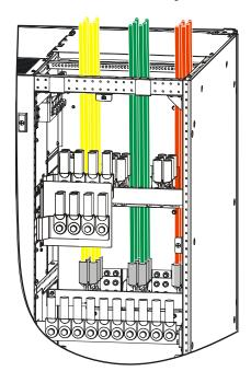
Figure 3-38 The PS800KVA AC output wiring diagram
