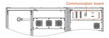
Figure 3-43 Communication board of PS800KVA
