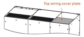
Figure 3-36 Top wiring cover plate position of PS800KVA
