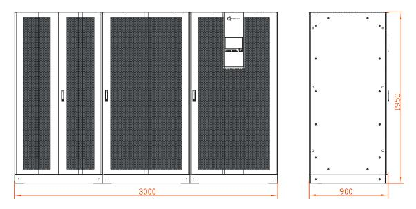
Figure 3-10 Size of PS1000KVAKR331200 (unit: mm)
