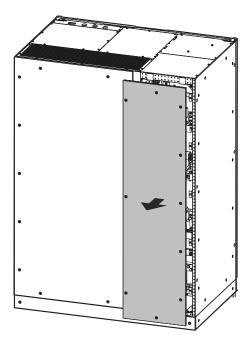
Figure 3-26 Dismantle wiring cover plates of PS500KVA, PS600KVA
