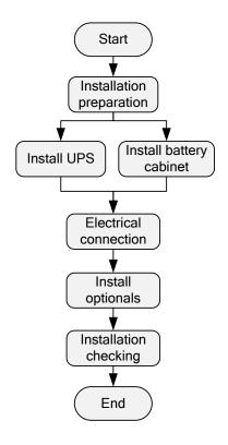
Figure3-1 UPS installation process
