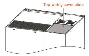
Figure 3-18 Top wiring cover plate position of PS300KVA, PS400KVA
