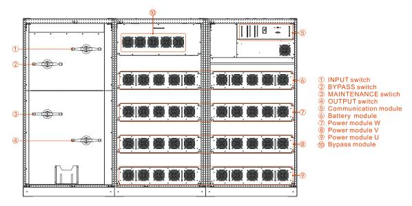
Figure 2-13 Structure layout of PS1000KVA, PS1200KVA (open door)
