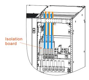
Figure 3-32 The PS500KVA PS600KVA battery wiring diagram
