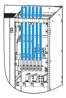
Figure 3-33 The PS500KVA PS600KVA output neutral wiring diagram
