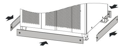
Figure 3-16 Install bottom cover plates
