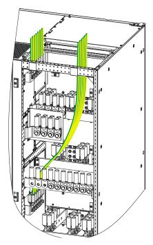
Figure 3-40 The PS800KVA grounding wiring diagram
