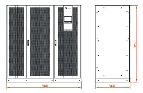
Figure 3-9 Size of PS800KVA (unit: mm)
