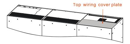
Figure 3-45 Top wiring cover plate position of PS1000KVA, PS1200KVA
