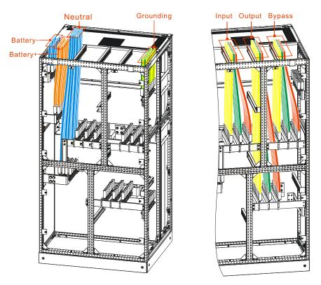
Figure 3-46 KR 331000, PS 1200 KVA wiring diagram
