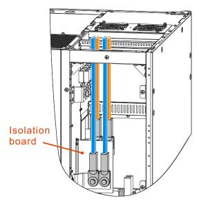
Figure 3-23 The PS 300 KVA, PS 400 KVA battery wiring diagram
