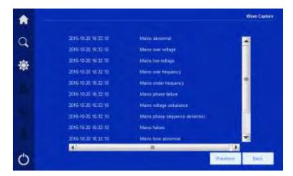
Figure 4-22 Corresponding fault details of fault time
