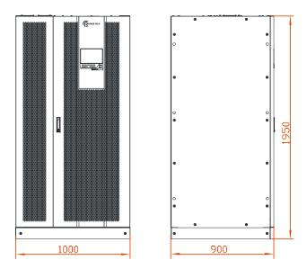
Figure 3-7 Size of PS300KVA, PS400KVA (unit: mm)
