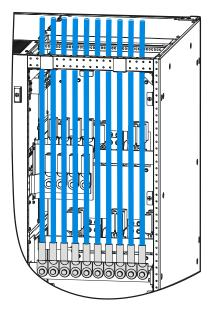
Figure 3-42 The PS800KVA output neutral wiring diagram
