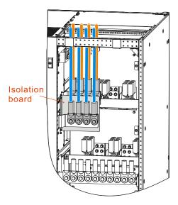
Figure 3-41 The PS800KVA battery wiring diagram
