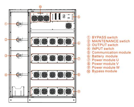
Figure2-11 Structure layout of PS500KVA, PS600KVA (open door)
