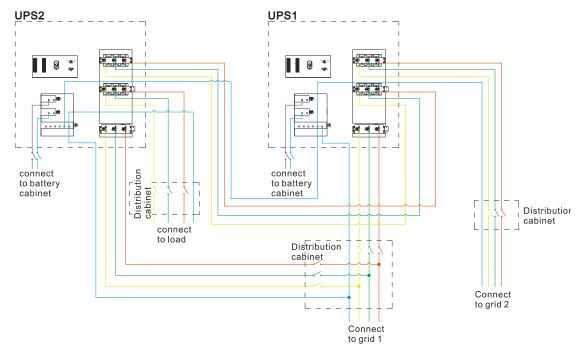
Figure 3-48 Wiring diagram of series system
