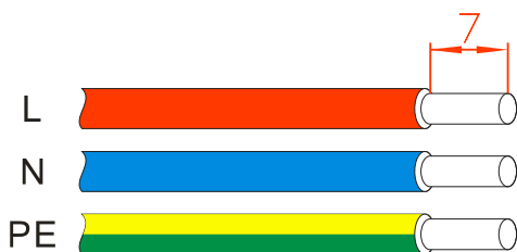
Figure3-34 Stripping diagram of AC output (unit: mm)
