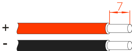
Figure3-26 Stripping diagram of DC input (unit: mm)
