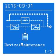
Figure4-6 Maintenance bypass output
