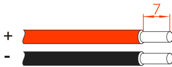
Figure3-35 Schematic diagram of stripping DC input wiring (Unit: mm)
