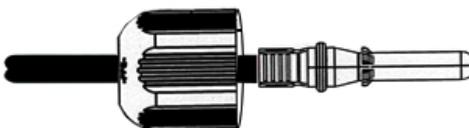
Figure3-17 Crimp the negative metal terminal
