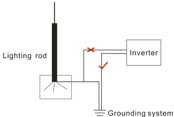
Figure3-11 The grounding of inverter
