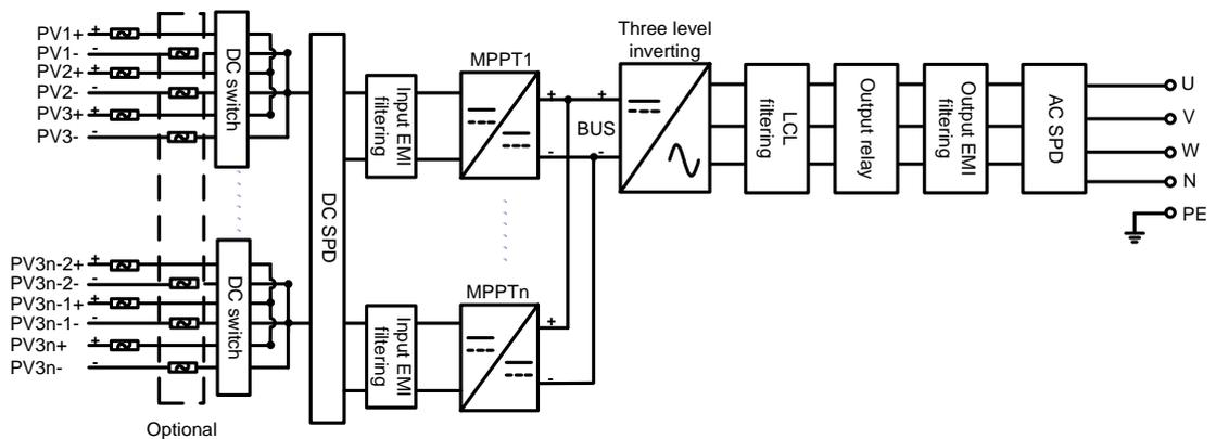
Figure2-6 Working principle diagram
