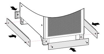
Figure 3-20 Install the bottom cover plates
