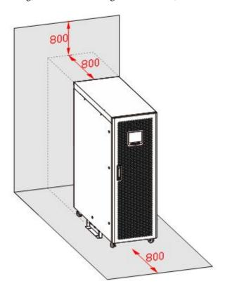
Figure 3-2 Installation space (unit: mm)
