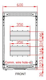
Figure 3-34 Wire inlet and outlet hole of down wiring of 160K, 200K
