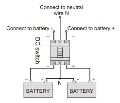
Figure 3-38 Battery wiring diagram
