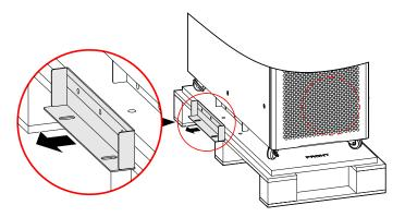
Figure 3-7 Dismantle the supporting plate of 60K, 80K, 100K, 120K
