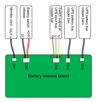
Figure 3-27 Illustration for terminal connection of battery release
