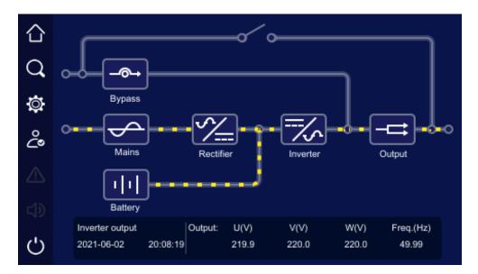
Figure 4-7 Mains inverter output
