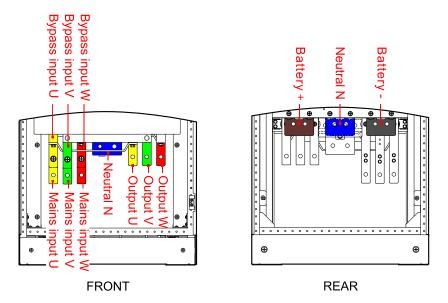
Figure 3-36 Wiring terminals bars diagram of 160K, 200K
