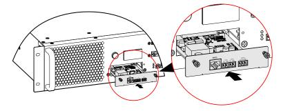
Figure 3-24 Install the expansion card
