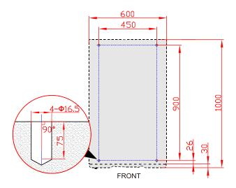
Figure 3-17 Bottom installation size (bottom view of pedestal)
