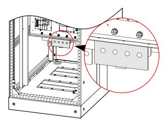
Figure 3-35 PE position of 160K, 200K
