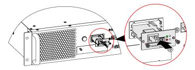
Figure 3-22 Install SNMP card
