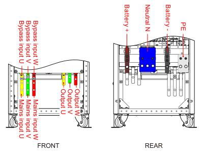
Figure 3-30 Wiring terminal diagram of 60K, 80K, 100K, 120K
