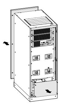
Figure 3-33 Remove the back and top wiring cover plate of 160K, 200K
