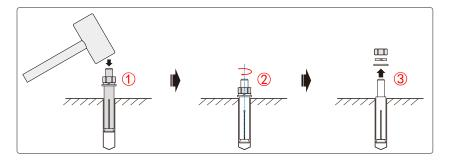
Figure 3-12 Install expansion bolts
