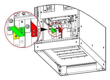
Figure 3-37 Short circuit terminal bars position of mains and bypass
