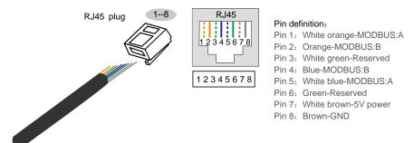
Figure 2-13 Pin definition of MODBUS
