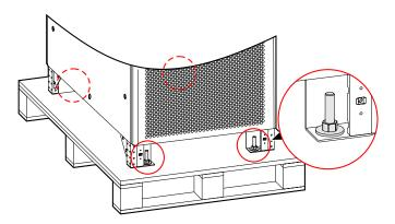
Figure 3-8 Bolts position of 160K, 200K
