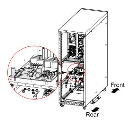
Figure 3-25 Installation position of PCB for 60K, 80K, 100K, 120K
