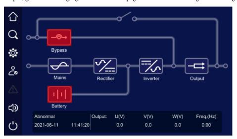
Figure 4-3 Abnormal protection, with no output
