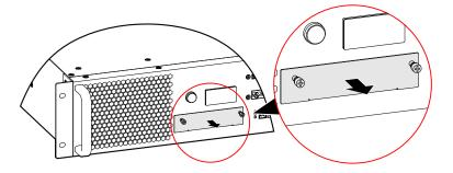
Figure 3-23 Dismantle the expansion card cover plate
