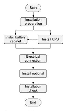
Figure 3-1 Installation procedure
