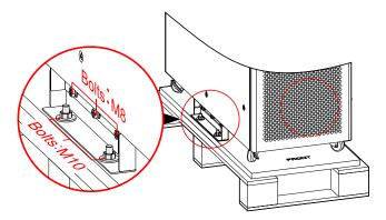
Figure 3-6 Dismantle the supporting plate of 60K, 80K, 100K, 120K
