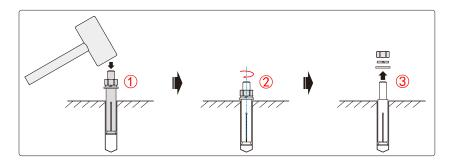
Figure 3-19 Install expansion bolts
