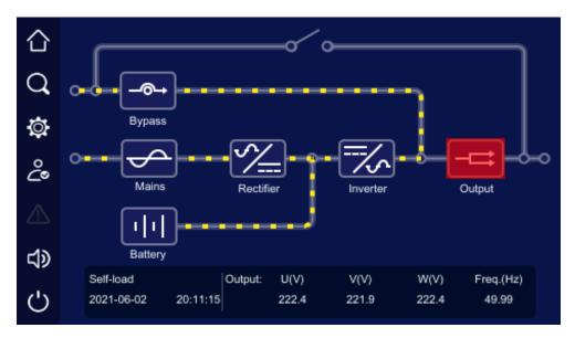
Figure 4-8 Grid-tied self-load running
