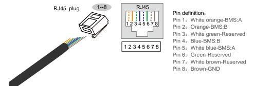
Figure 2-19 Pin definition of BMS port
