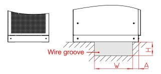
Figure 3-15 Trunking diagram
