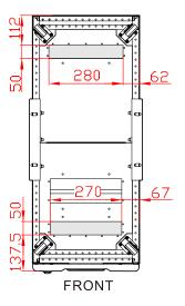
Figure 3-29 Down wiring holes diagram of 60K, 80K, 100K, 120K
