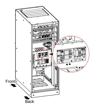
Figure 3-26 Installation position of PCB for 160K, 200K
