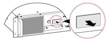
Figure 3-21 Dismantle the SNMP card cover plate
