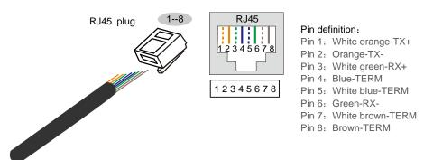
Figure 2-16 Pin definition of NETWORK port
