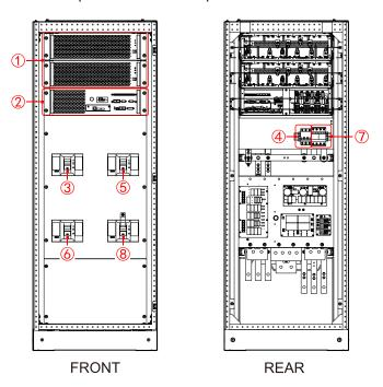
Figure 2-7 Structure layout diagram of 160K, 200K (open the door)
