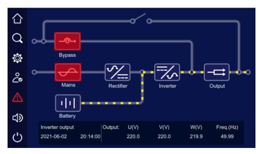
Figure4-6 Battery inverter output
