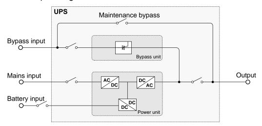
Figure 2-1 Work principle diagram
