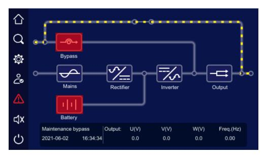
Figure 4-11 Maintenance bypass output
