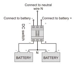
Figure 3-32 Battery wiring diagram
