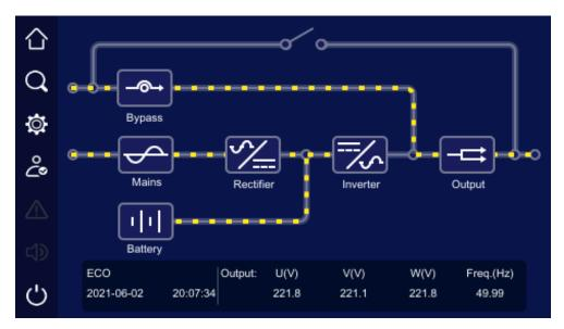
Figure4-9 ECO bypass output
