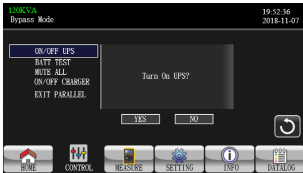
TURN ON UPS
