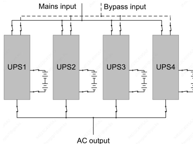
Make sure each UPS input switch is in “off” position and there is no any output from each UPS connected. Battery groups can be connected separately or in parallel, which means the system itself provides both separate battery and common battery.
