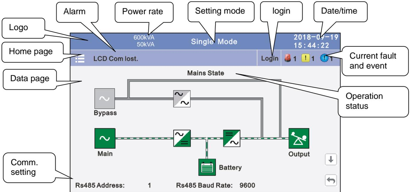
**4.3.1 Datas:** Displays the flow state of UPS work, and quickly enters real-time data by clicking on the block.
