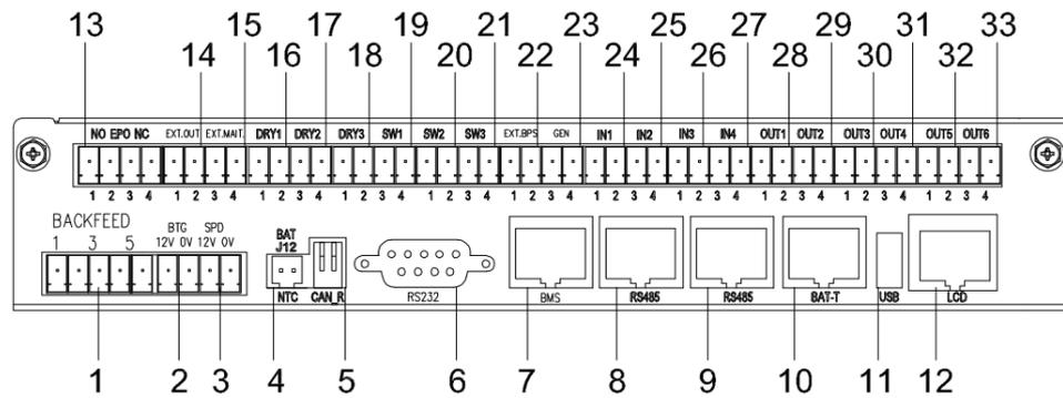
(1) BACKFEED: Bypass backfeed singnal input port, PIN1\_common, PIN3\_NO, PIN5\_NC
