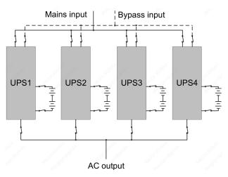
Make sure each UPS input switch is in "off" position and there is no any output from each UPS connected. Battery groups can be connected separately or in parallel, which means the system itself provides both separate battery and common battery.
