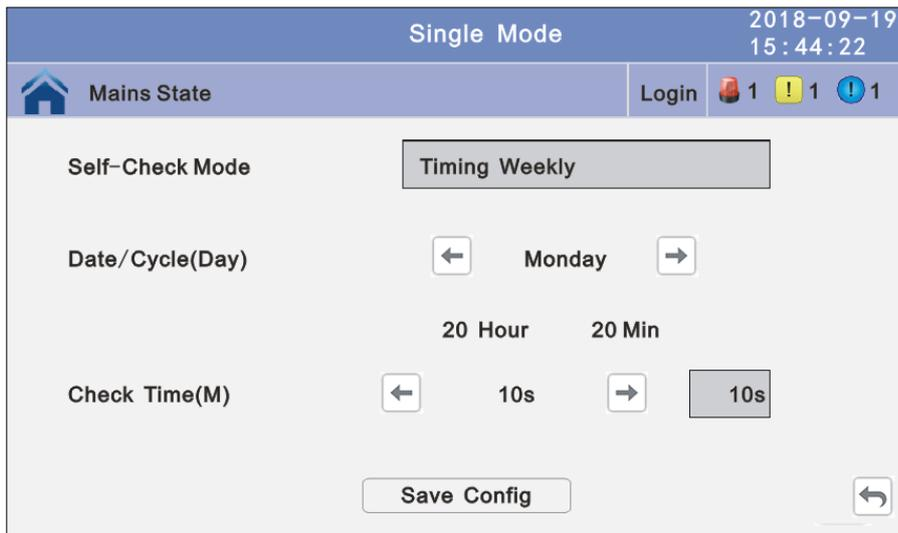
**4.3.5.2.3 Timing Cycle mode:** modify the cycle date and check time (10S (default), 10min, EOD).
