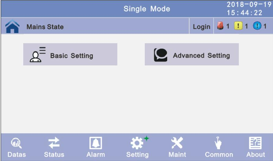
**4.3.4.1 Basic Setting:** Click basic setting, enter by input the correct password. The user password is "111111".
