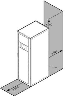
Please place the UPS in a clean, stable environment, avoid the vibration, dust, humidity, flammable gas and liquid, corrosive. To avoid from high room temperature, a system of room extractor fans is recommended to be installed. Optional air filters are available if the UPS operates in a dusty environment.
