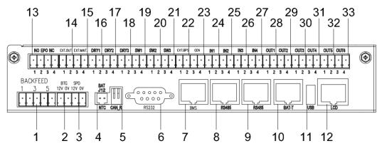
Definition of input and output ports
