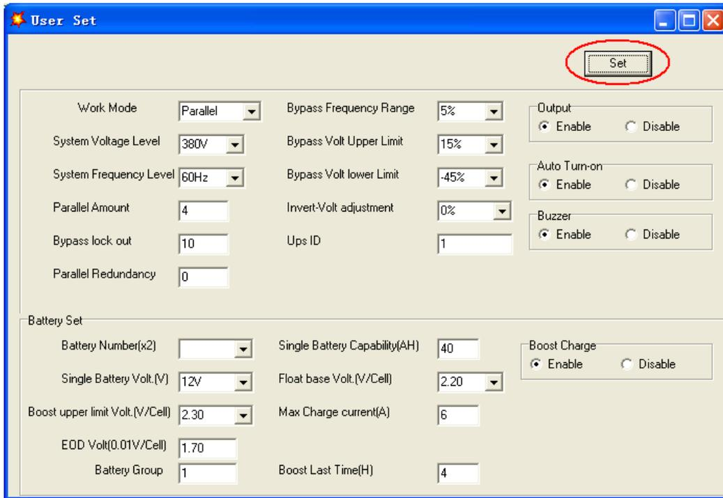
◆At the window of “Data Set”, click “Work Mode”, choose “Parallel” for the value, then click “Set” as shown in below picture. If the UPS sounds a “beep”, that means the setting is correct.
