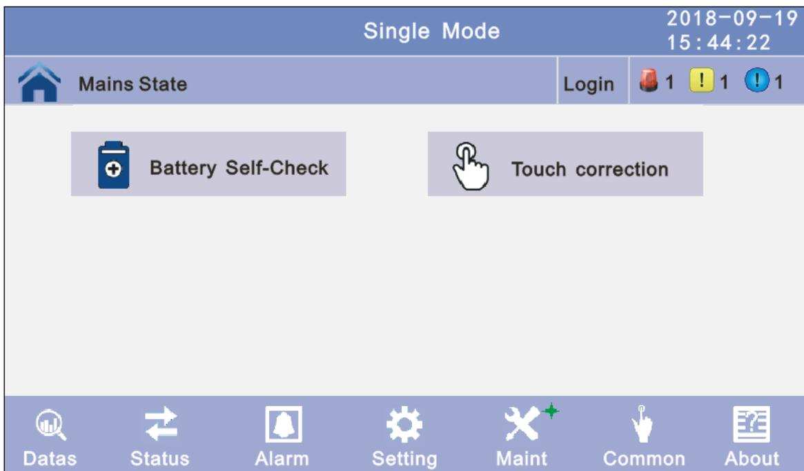
**4.3.5.1 Battery Self-Check:** can select check by Timing Daily, Timing Weekly, Cycle mode. The default value is Timing Self-Check Close.
