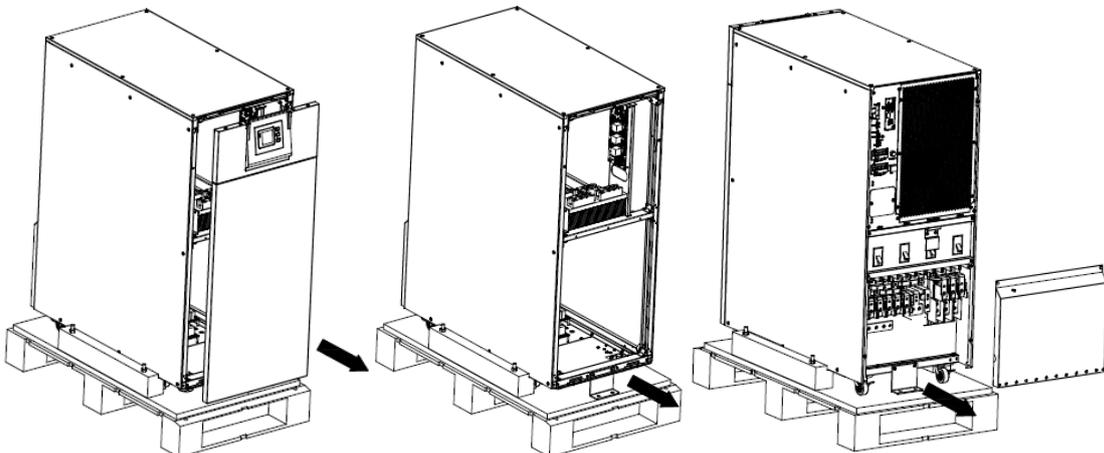
**Step 8** Remove the front panel and rear panel to remove the L-shaped bracket and the plates at the left and right side of the UPS that secures the cabinet and the pallet, and secure the sliding
