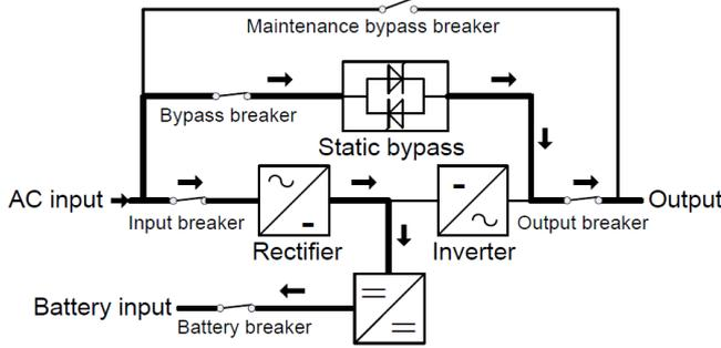
**DUAL INPUT: Mains Input and Bypass Input**
