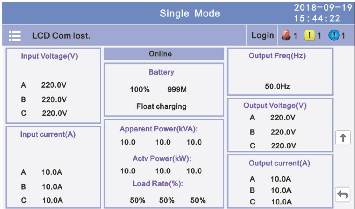
**4.3.2 Status:** View the voltage and current of the main, bypass, output, battery (can also be entered through by real-time data block), view the status of the switches, dry contacts, through clicking on the block, enter the corresponding data window.
