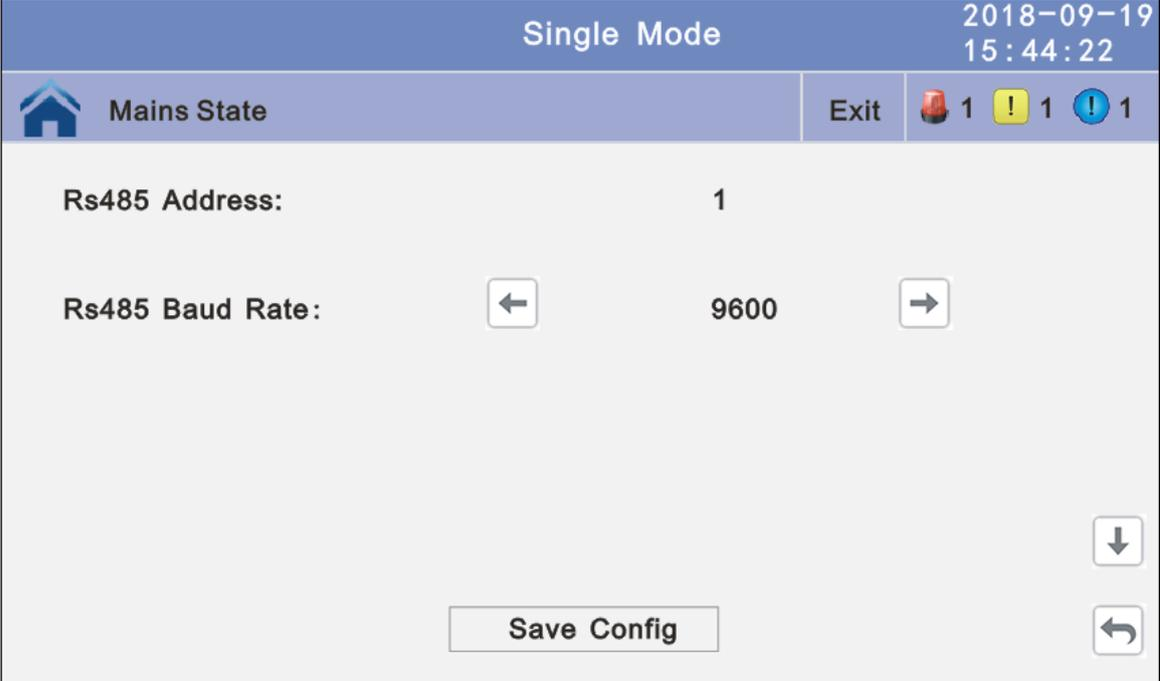
**4.3.4.2 Advanced Setting:** Click advanced setting, enter by input the correct password. The user password is "191210".
