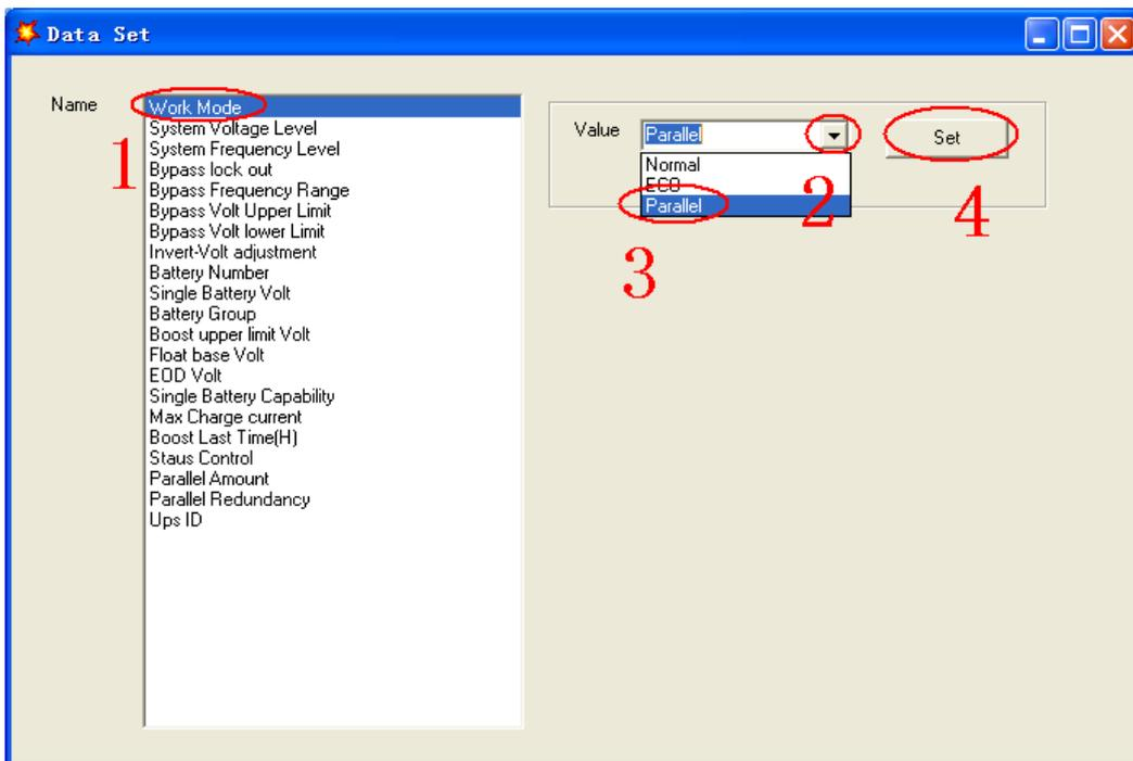
◆At the window of “Data Set”, click “Ups ID”, write a value for the parallel UPS ID at the right side, such as “1”, then click “Set” as shown in below picture. If the UPS sounds a “beep”, that means the setting is correct.
