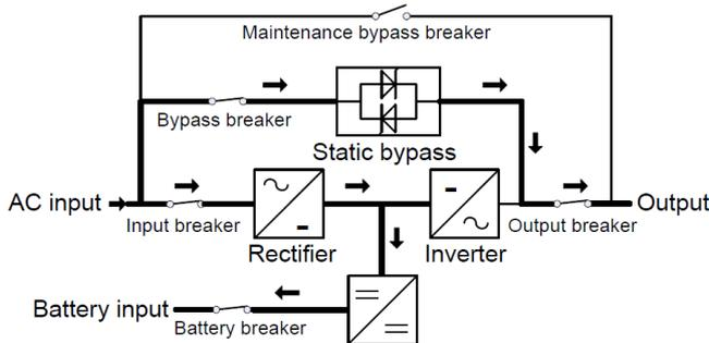
**DUAL INPUT: Mains Input and Bypass Input**
