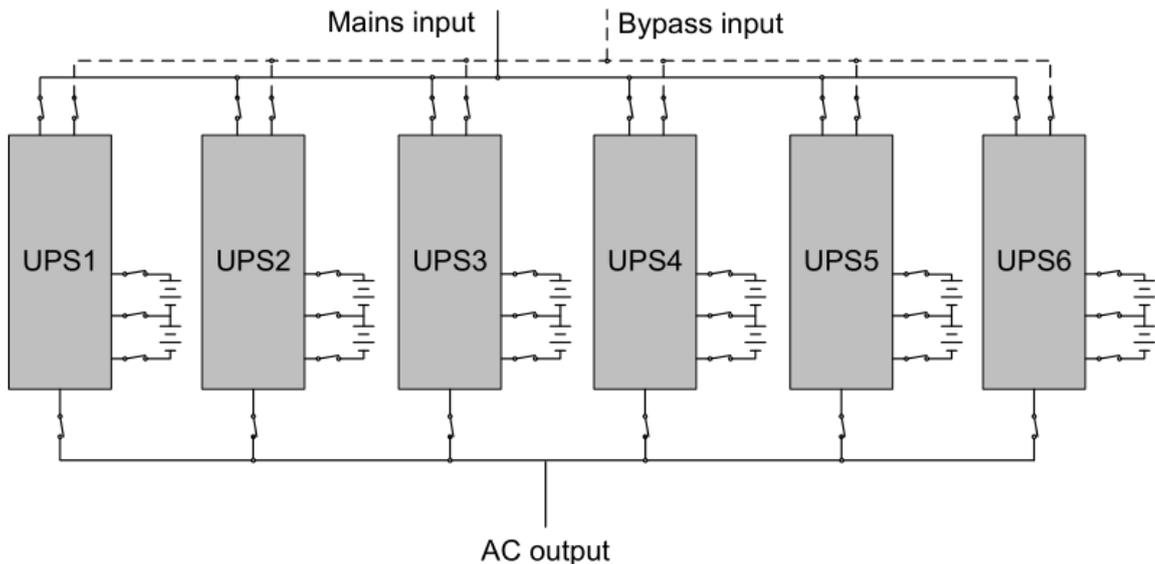
Make sure each UPS input breaker is in “off” position and there is no any output from each UPS connected. Battery groups can be connected separately or in parallel, which means the system itself provides both separate battery and common battery.
