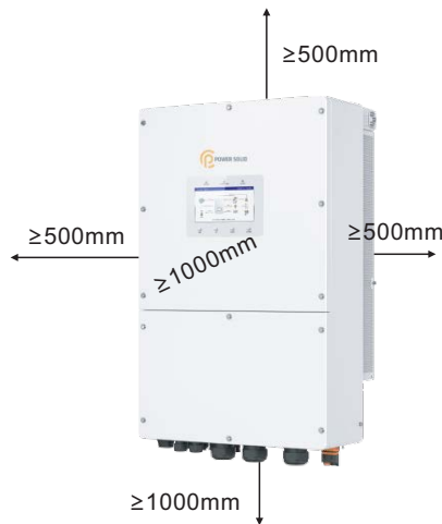
Figure 3.5 Inverter Mounting Clearances
